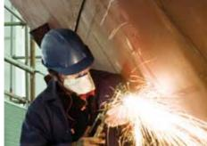
a perfect weld can be affected by the generic type of shopprimer and dry film thickness. The introduction of automatic welding (MIG/MAG) has increased productivity compared to stick welding (MMA or SMAW). Besides being more productive, automatic welding results in less exposure of the welders to any toxic welding fumes.
